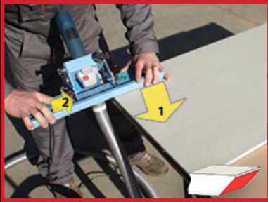
Vacuum port for use when dry cutting
