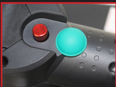
Rubber button cover protects against dust & moisture
