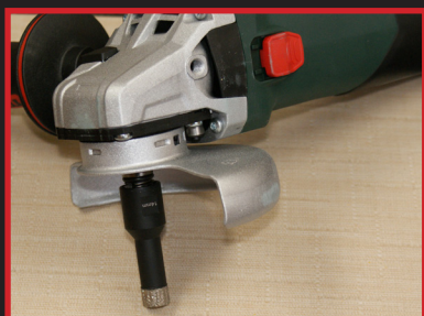
Use with right angle grinder with 5/8"- 11 Thread
