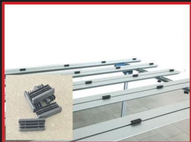
Spacers to raise work piece for cutting or drilling
