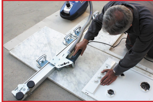
Shown with optional Kera-Flex accessory for plunge & L cuts
