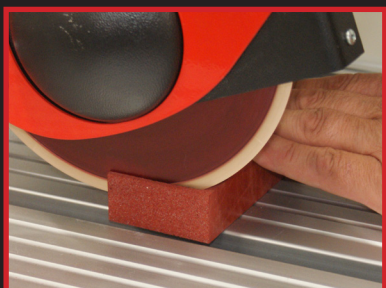
Cut into the stone to sharpen diamond products
