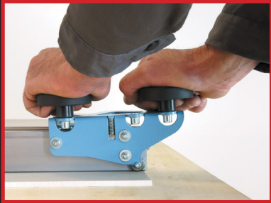
Two-handed scoring provides optimum pressure
